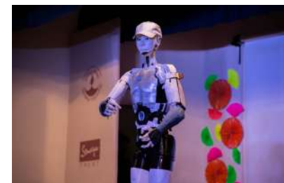
Robyn Inmoov First Open Source 3D printed life-size robot
