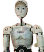
Robyn Inmoov First Open Source 3D printed life-size robot
